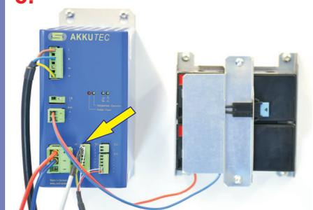
Wiring of the temperature sensor
