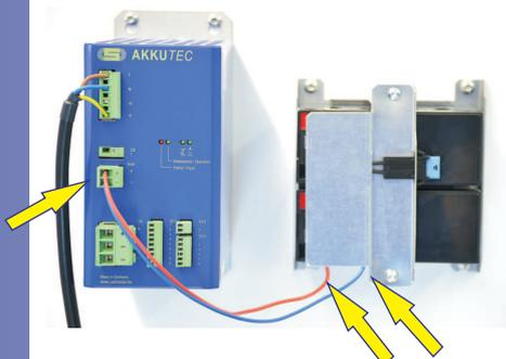
Connect the battery to the batter connector of the AKKUTEK
