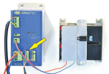
Connect the RS232 interface cable (Art. Nr. PSDP0324G0100X)
